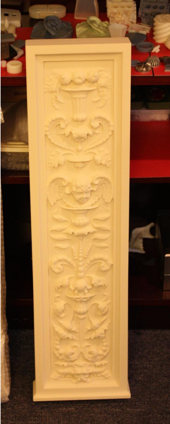
Finished piece of the foyer carving made from CNC cut foam.
