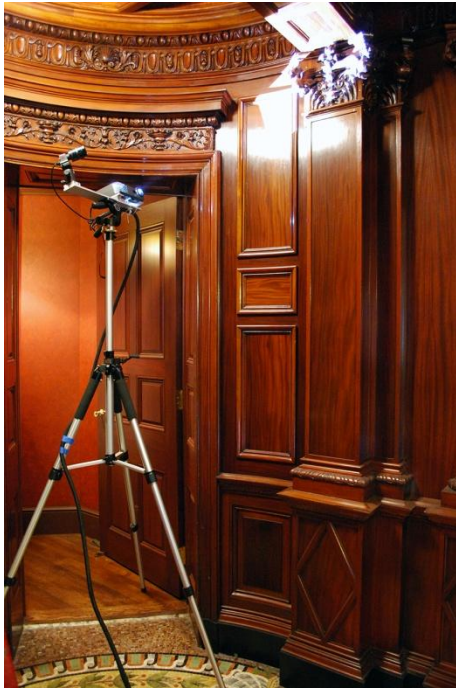
Scanning the flying monkey capital. Note the dark, glossy wood finish did not need to be sprayed with a white powder for 3D scanning.
